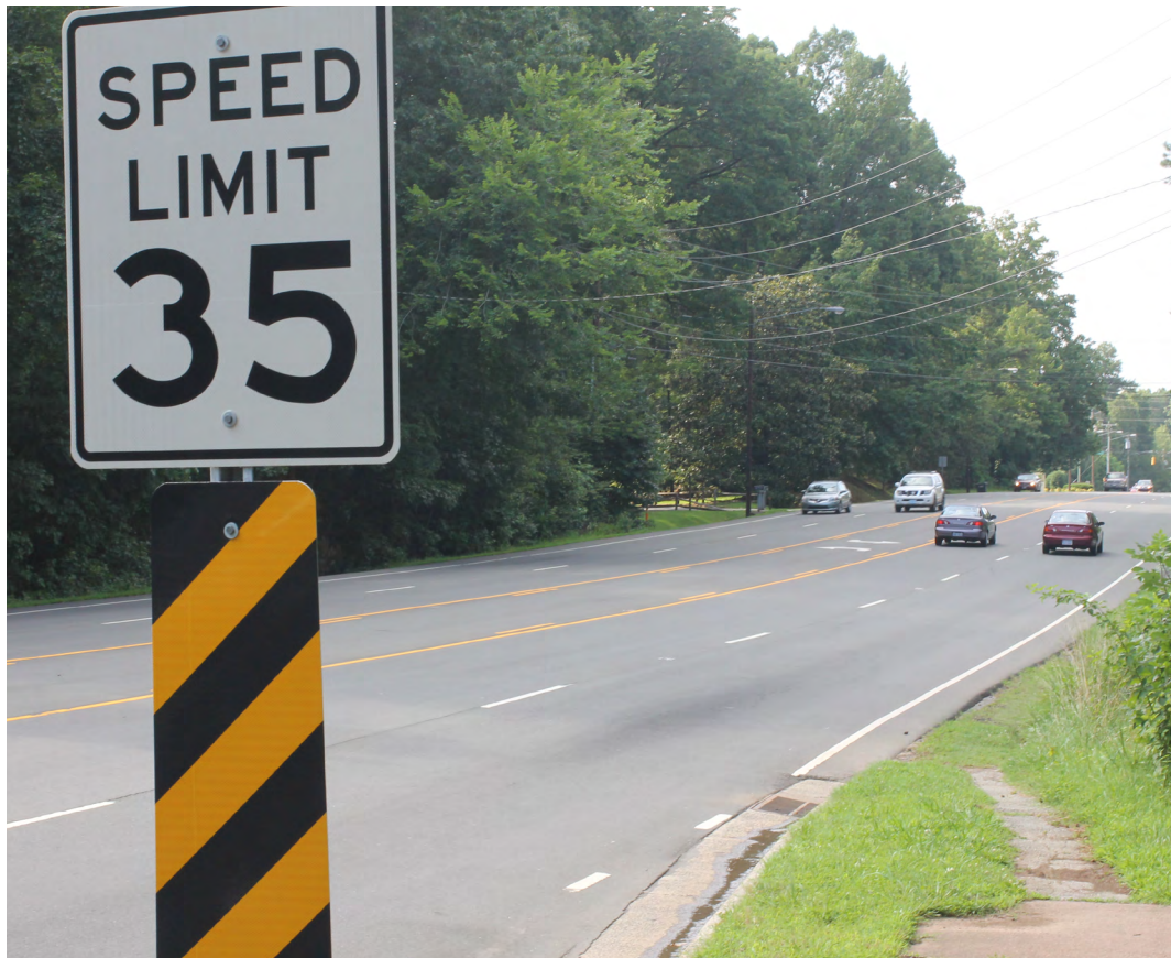
The intended speed of this road is 35 miles per hour, but the wide design of the road and the number of lanes leads drivers to drive much faster.
