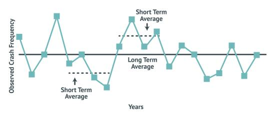
FIGURE 4-4: Chart to illustrate RTM phenomenon (Source: HSIP Manual, 2010)
