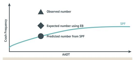
FIGURE 4-5: Schematic to illustrate the empirical Bayes method (Source: HSIP Manual, 2010)
