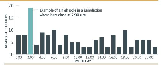
FIGURE 4-9. Example of "high pole" in crash data (Source: NCHRP Report 501)
