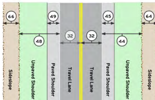
FIGURE 3-2: This image from the FHWA Model Inventory of Roadway Elements (v. 1.0) illustrates roadway elements.
